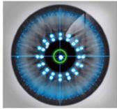
The system projects 32 concentric light points onto the cornea, aligning reflections for high-precision, repeatable calculations.
